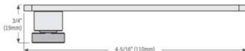
Ball bearing single roller, stainless steel
