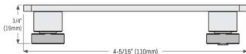
Ball bearing double roller, stainless steel
